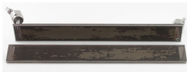
Fig. 10 Microreactor after experiments with galactose hydrogenation
